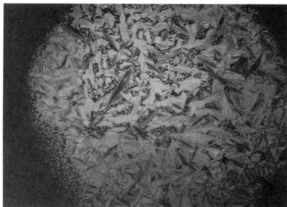
Figure 6. Optical micrographs of the mesophase textures for polymer 13 ( \times 75 ): (A) Ch (200 °C); (B) Sa (130 °C).
